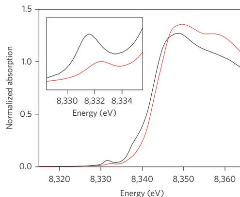
**Figure 3 | Ni K-edge X-ray absorption spectra of 1 (red) and 2 (black).** The inset shows the expanded pre-edge region. The Ni K-edge X-ray absorption spectrum of **2** was reported previously in ref. 18. Owing to large differences in the beamline optics, cryostat temperatures, and detection methods, the data were re-measured in the present study for accurate comparison of **1** and **2** under identical conditions.
