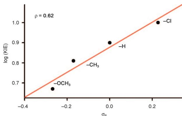
Figure 3. Plot of  $\log(KIE)$  of 1-Y against  $\sigma_p$  of the substituents of *p*-Y-PyO in the oxidation of xanthene by  $[(tmp)^+Fe^{IV}(O)(p\text{-}Y\text{-}PyO)]^+$ .
