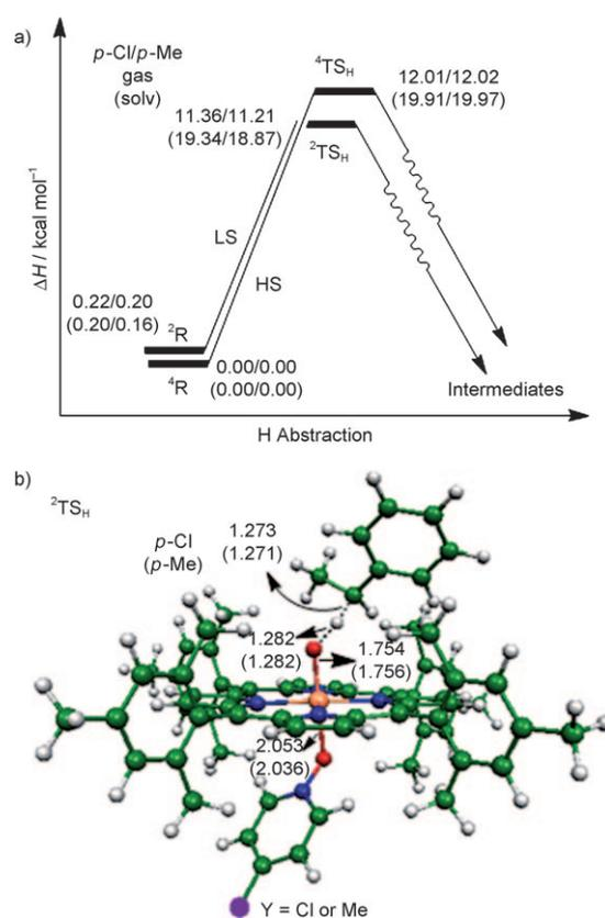
Figure 6. a) Reaction profiles and b) TSs on doublet (LS) and quartet (HS) of H-abstraction of ethylbenzene by  $[(\text{tmp})^+\text{Fe}^{\text{IV}}(p\text{-Y-PyO})]^+$ .
