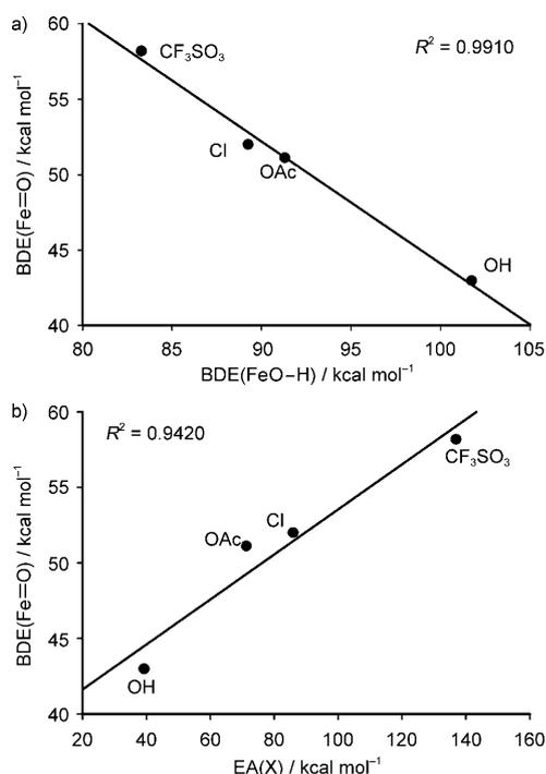
Figure 5. a) BDE of  $\text{Fe}=\text{O}$  versus BDE of  $\text{FeO}-\text{H}$  (the respective bond dissociations to the most stable spin states). b) BDE of  $\text{Fe}=\text{O}$  versus electron affinities of axial-ligand radicals.
