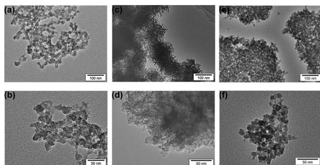
**Fig. 10** TEM images of nanoparticles formed during the photocatalytic water oxidation with (a and b) **1**, (c and d) **2** and (e and f)  $\text{Co}(\text{NO}_3)_2$  in a buffer solution (pH 9) containing  $[\text{Ru}(\text{bpy})_3]^{2+}$  (0.50 mM) and  $\text{Na}_2\text{S}_2\text{O}_8$  (10 mM).
