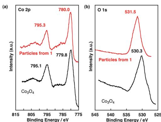
**Fig. 11** X-ray photoelectron spectra of particles derived from **1** (red) and  $\text{Co}_3\text{O}_4$  (black) as a reference compound in the energy regions of (a) Co 2p and (b) O 1s. The binding energy of each element was corrected by the C 1s peak (284.6 eV).
