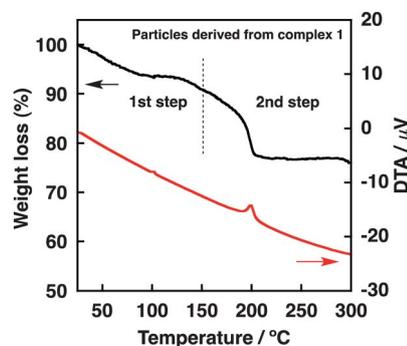
**Fig. 12** TG/DTA data for nanoparticles derived from complex **1** (TG curve: black, DTA curve: red). The temperature increased from 25 °C to 300 °C with a ramp rate of 2 °C min<sup>-1</sup>.
