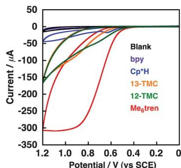
**Fig. 7** Cyclic voltammograms of a buffer solution (pH 8.0, 50 mM; black line) containing ligands of **1–4** (4.0 mM); bpy (purple line),  $\text{Cp}^*\text{H}$  (blue line), 13-TMC (yellow line), 12-TMC (green line) and  $\text{Me}_6\text{tren}$  (red line) at a scan rate of  $100 \text{ mV s}^{-1}$ .
