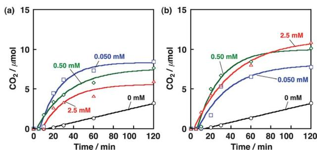
**Fig. 8** Time courses of CO<sub>2</sub> evolution under photoirradiation (Xe lamp,  $\lambda > 420$  nm) of a buffer solution (2.0 mL, 100 mM borate, pH 9.0) containing [Ru(bpy)<sub>3</sub>]<sup>2+</sup> (0.50 mM), Na<sub>2</sub>S<sub>2</sub>O<sub>8</sub> (50 mM) and a cobalt precatalyst of (a) Co(NO<sub>3</sub>)<sub>2</sub> or (b) **1** at concentrations of 0 mM (black circle), 0.050 mM (blue square), 0.50 mM (green diamond) and 2.5 mM (red triangle).
