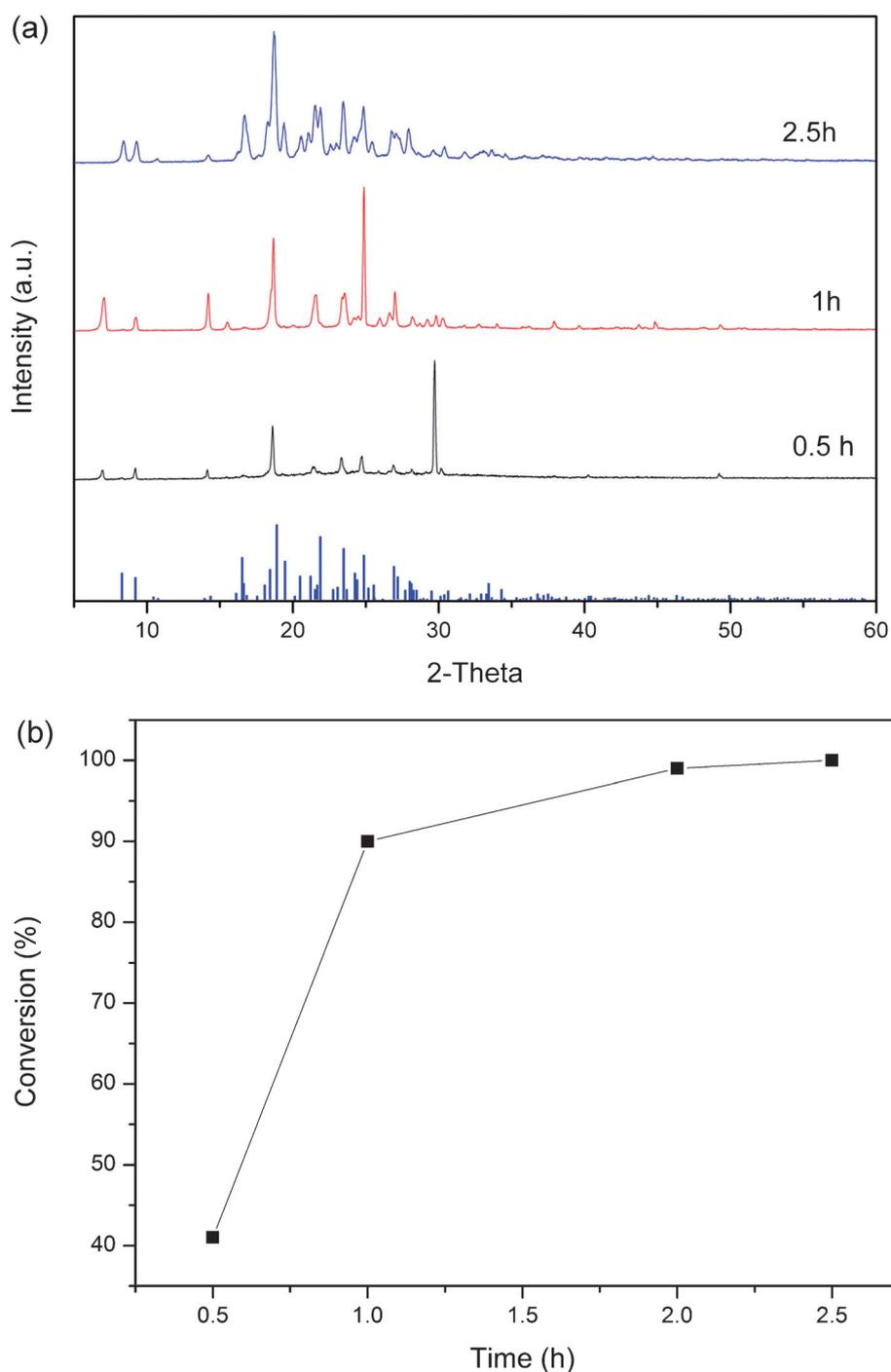
**Figure 2.** (a) Powder XRD patterns of the products obtained by grinding a mixture of **2a** and the aromatic aldehyde (**3a**, Table 1, entry 1) at intervals of 30 min, 1 h, and 2.5 h at 25°C. The vertical bars at the bottom of the spectrum correspond to the theoretical diffraction peaks of **4aa**. (b) Yields of **4aa** as a function of reaction time were determined by  $^1\text{H}$  NMR spectroscopy.
