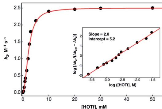
Fig. 4 Dependence of the second-order rate constant,  $k_2$ , for the oxidation of *para*-CN-thioanisole by **3** (0.50 mM) on  $[\text{HOTf}]$  (0–50 mM) in  $\text{CF}_3\text{CH}_2\text{OH}\text{--}\text{CH}_3\text{CN}$  ( $v/v = 1 : 1$ ) at 273 K. Inset shows a plot of  $\log[\Delta k_2/(\Delta k_{2,0} - \Delta k_2)]$  vs.  $\log[\text{HOTf}]$ , where  $\Delta k_{2,0}$  is the full change of second-order rate constant.
