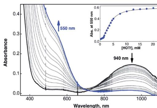
Fig. 2 UV-vis spectral changes observed in the titration of **1** (black bold line) with HOTf. HOTf (0–20 mM) was added incrementally into the solution of **1** (0.50 mM) in CF<sub>3</sub>CH<sub>2</sub>OH-CH<sub>3</sub>CN (*v/v* = 1 : 1) at 273 K. Inset shows the spectral titration monitored at 550 nm (blue circles) due to the formation of **3**.
