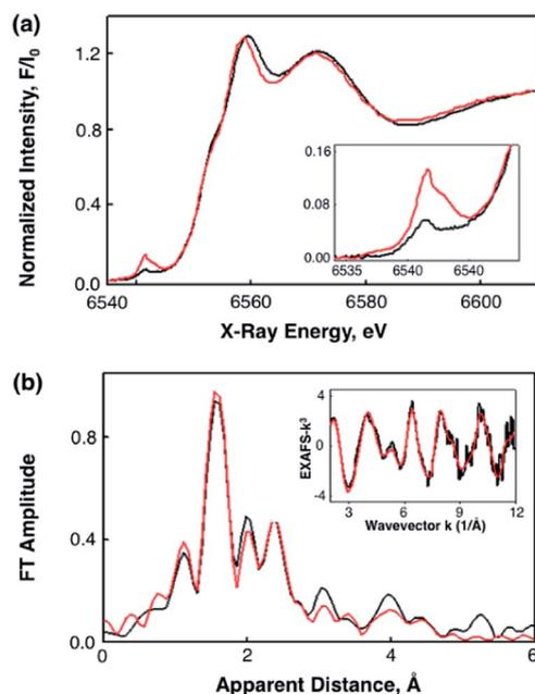
Fig. 3 (a) Normalized Mn K-edge XANES of **1** (red line) and **3** with 30 mM of HOTf (black line). Inset shows magnified pre-edge features. (b) Non-phase-shift corrected Fourier transforms (black line) and the corresponding Mn K-edge EXAFS data (inset; black line) for **3**. Fits (red lines) were performed in the range of  $k = 2\text{--}12 \text{ \AA}^{-1}$ .
