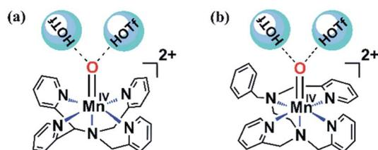
Fig. 1 Schematic drawing of the chemical structures of [(N4Py)Mn<sup>IV</sup>(O)]<sup>2+</sup> (a) and [(Bn-TPEN)Mn<sup>IV</sup>(O)]<sup>2+</sup> (b) species binding two HOTf molecules.
