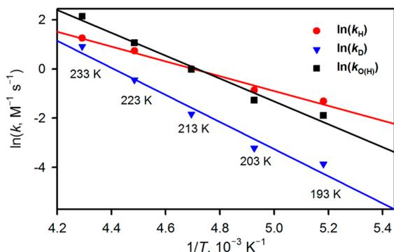
**Figure 2.** Arrhenius plots of the rate constants of epoxidation ( $k_{O(H)}$ ) and hydroxylation of cyclohexene- $d_{10}$  ( $k_H$ ) and cyclohexene- $d_{10}$  ( $k_D$ ) by  $[(TMP^{*+})Fe^{IV}(O)(Cl)]$  (**1**) in  $C_3H_7CN$ .
