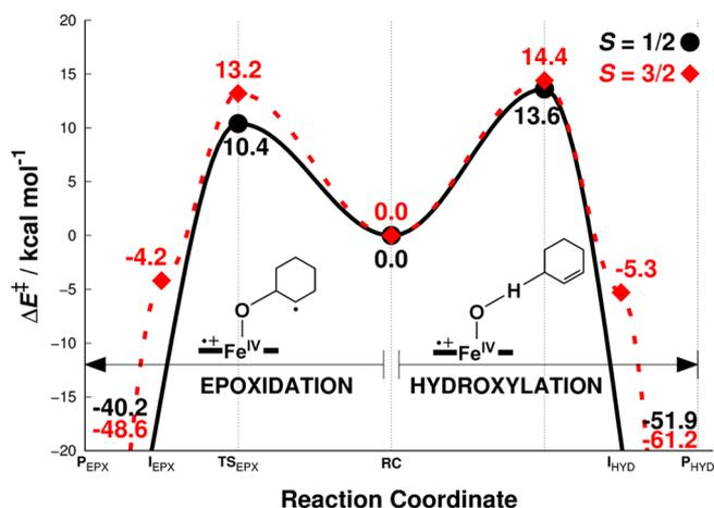
**Figure 3.** DFT-calculated reaction energy barriers for the oxidation reactions of cyclohexene by **1** at the B3LYP/LACVP3P+\*//LACVP level including dispersion and solvent effects.
